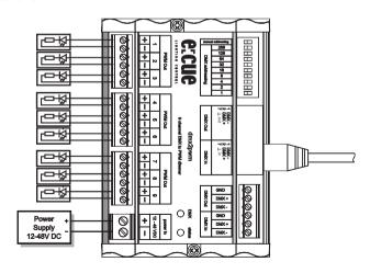
The advantage of the above shown type of connection is the reverse supply protection of all LED fixtures and the dimmer itself. Alternatively it is also possible to connect LED fixtures as shown in the figure at the right side.
